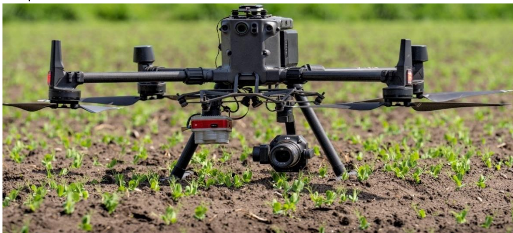
Figure 7 Drone DJI Matrice M300 RTK with MicaSense Altum and DJI Zenmuse P1 camera.
